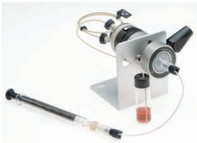
Figure 6. Sample loading by suction through a dip tube. A Model 7252 2.5 mL syringe is shown connected to the valve needle port using a Model 9125-076 Needle Port Adapter.
