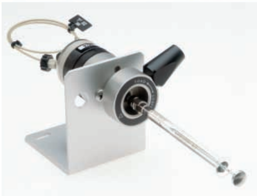
Figure 5. Sample loading by dispensing from a syringe. The sample injection valve is shown mounted to a Model 7160-010 Valve Angle Bracket. A Model 7200 2.5 \mu\text{L} syringe is shown.
