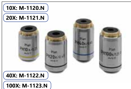
IOS (infinity corrected) Phase Contrast Plan Objectives
