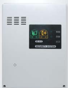
• Remote Wire/Wireless Alarm System (Optional) - Set to be activated when the temperature inside the chamber goes up to -65 °C. - Main controller signals to RWAS, if connected, at the alarm status, and then RWAS makes phone calls or send messages. - User could set and store multiple phone numbers and alarm statements.
