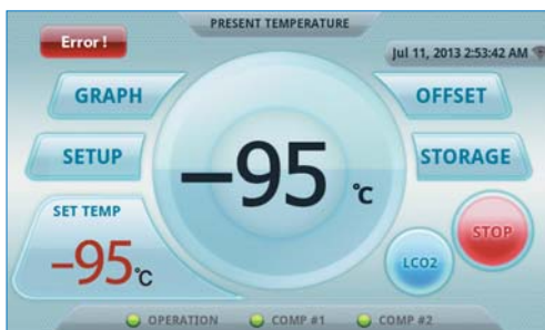
7" Full Touch Screen TFT LCD (Smart-Lab™ Controller)
