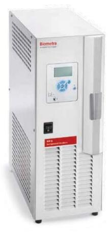
In the front panel integrated fill and drain ports, as well as the level indicator, ensure easy accessibility and trouble-free operation. The small internal reservoir eliminates evaporation and provides quick tempering. The powerful pump (max flow rate 7.5 l/min or 15 l/min) ensures an excellent temperature uniformity and an efficient heat exchange with external objects. Thus, a high degree of temperature accuracy is attainable.
